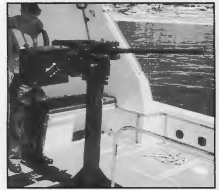
GA1 20x82mm automatic cannon shown in one of its naval applications: a pedestal deck mount on a light boat.
